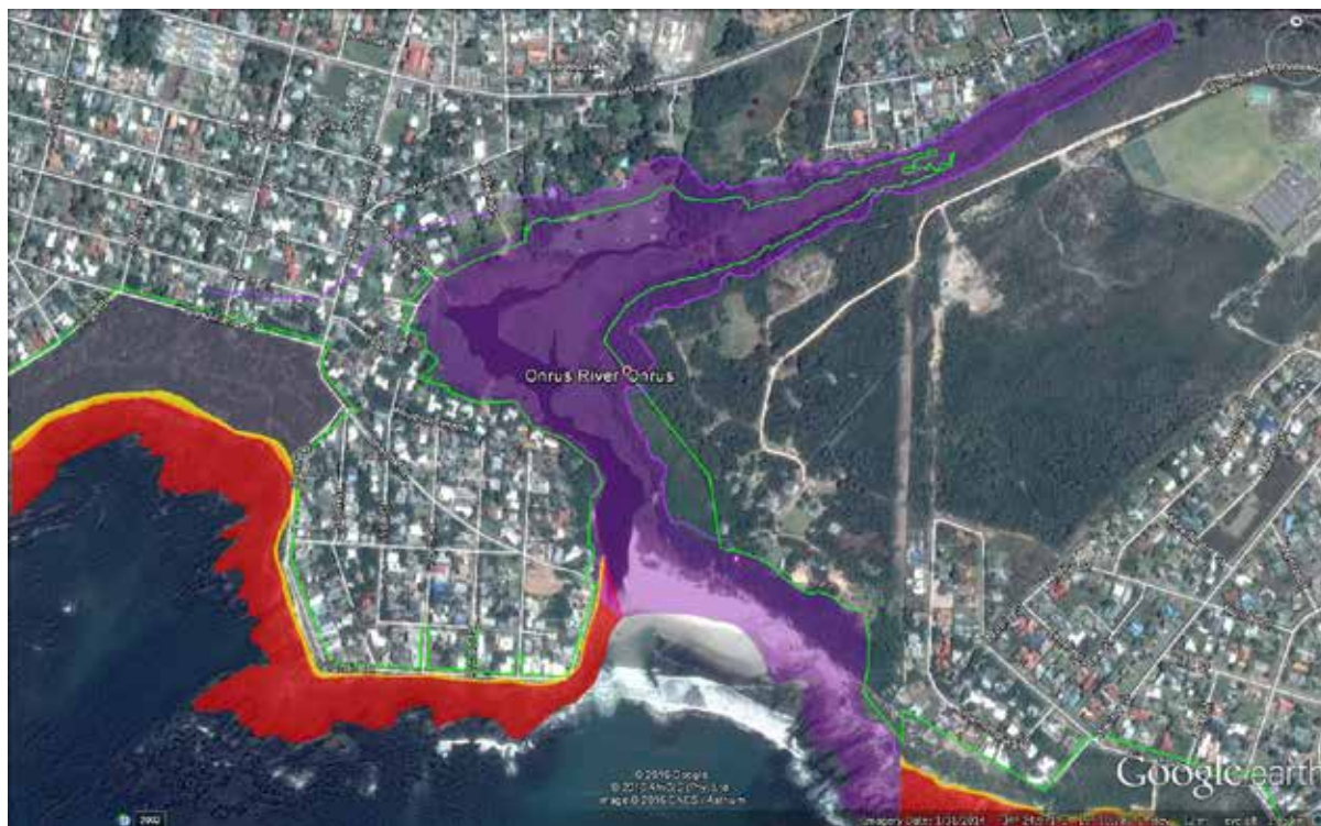
Figure 23 The green line represents the Coastal Management Line and the purple line the 10 m above mean sea level contour line that partially delineates the Estuarine General Risk Overlay Zone. The purple area shows the general risk zone in rural areas (1:100 year risk zone) that has been adapted for the Onrus Estuaries by incorporating the 10 m amsl line. The grey area outlines development islands within the 1:100 year risk zone. The red, orange and yellow areas represent the high (1:20), medium (1:50) and low (1:100 year) risk zones for the urban/developed areas respectively (Source: DEA&DP 2016).
