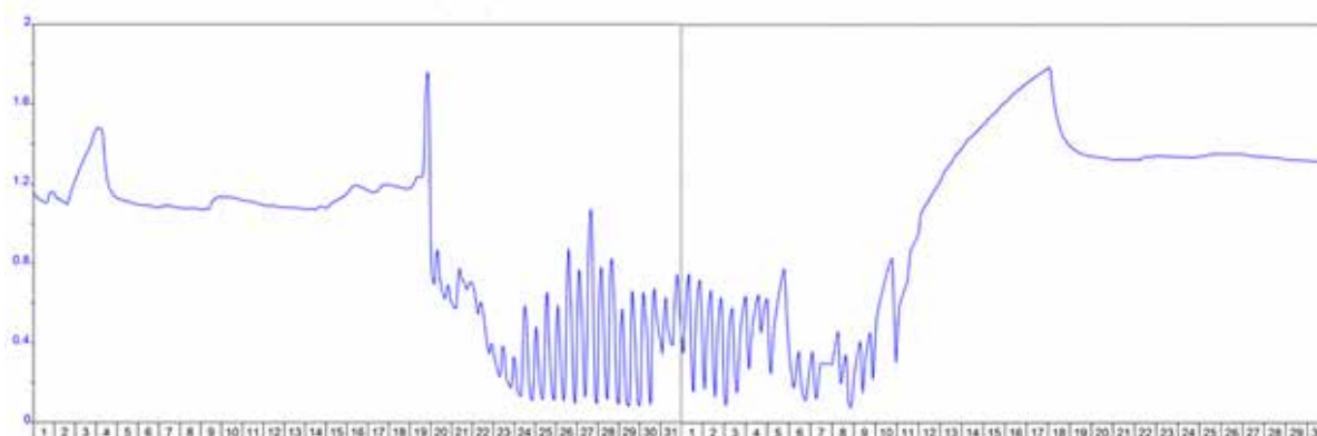
Figure 11 Data from the Onrus Lagoon water level gauge plotted for one-hour intervals for the period 1 October to 30 November 2012. The lagoon breached naturally on 19 October 2012 following heavy rainfalls. First the water level increased, then the lagoon drained, after which tidal fluctuations were evident for a short period before the mouth closed once more (Source: Department of Water and Sanitation).
